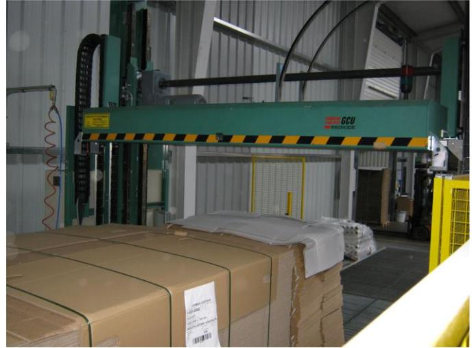
A Signode GCU 2500 compression machine in operation strapping palletized corrugated products. The integrated machine turntable enables loads to also be cross-strapped. Depending on the type of product the loads can be compressed before strapping with compression levels of up to 25.000 N. The press uses as standard 9 mm Tenax®
