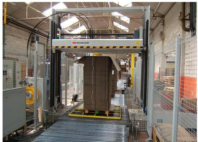
The GCU 2800 press can strap pallets and pallet-less loads for high throughputs, and ensures high machine uptime. GCU 2800 presses are equipped with top-edge protection applicators as standard and can be further equipped with bottom edge-protection applicator magazines. The units apply standard 600 - 800 mm long and 250 - 300 mm wide corrugated strips..
