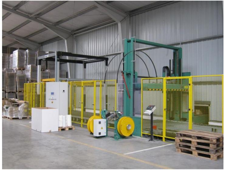
A Signode supplied packaging line composed of GCU 2500 corrugated compression machine, pallet handling system Octopus 2800 wrapping machine and complete machine guarding system including a light guard system.
