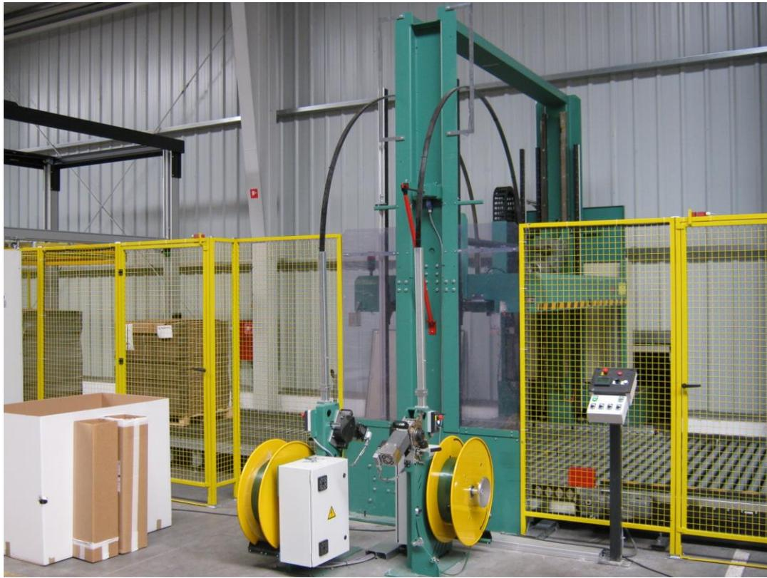
GCU Compression strapping using the unique modular MH strapping heads
