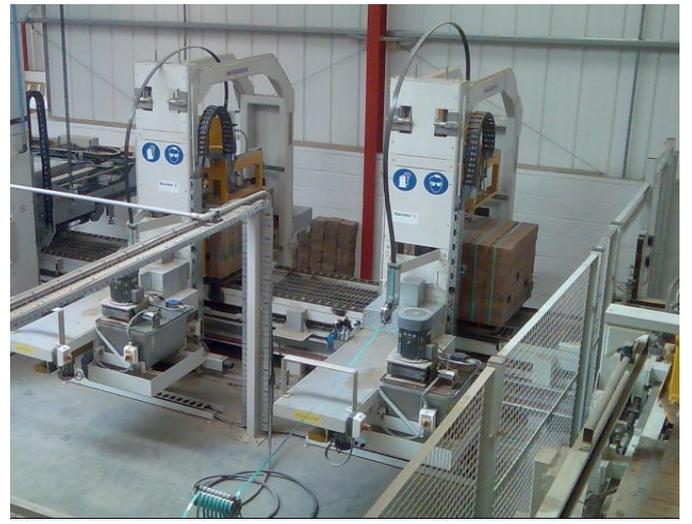
Tandem vertical machines in a high throughput line with automatic strap feed-up to the Z-20 heads
