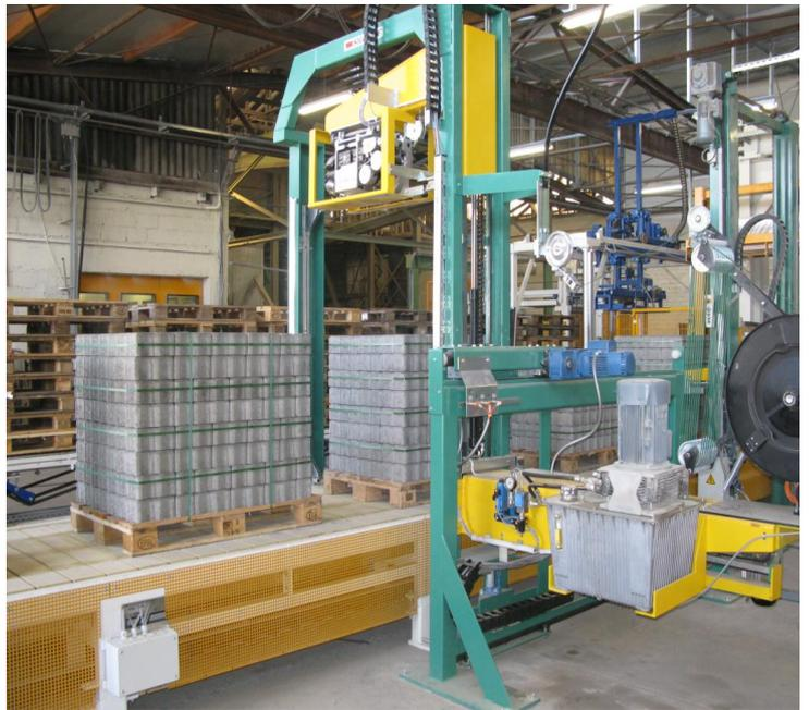
A combination of a vertical MH strapping machine with upstream MH-H horizontal model and a top sheet applicator unit provide the customer with a fully automatic, high-speed flexible end-of-line packaging solution. The interchangeable modules can be rotated around the plant machines in various MH machines for maximum equipment availability at lowest possible cost
