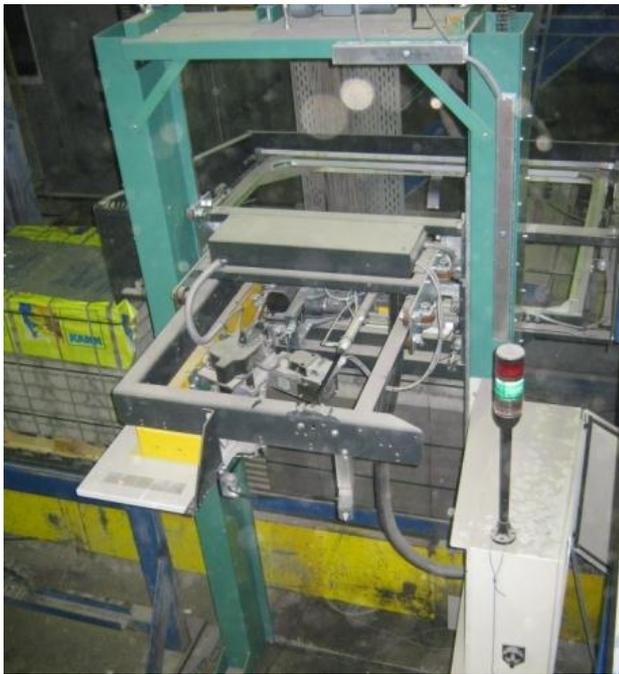
The MH-H horizontal machine featured here shows the separate feeder and sealer modules which make the MH system so reliable and durable. Even in such extreme conditions with aggressive dust particles the modules continue to work efficiently and reliably. The units apply consistently high strap tension for optimum load securement for storage and transport
