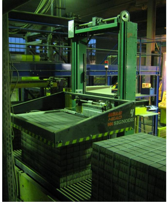
Signode modular MH-H horizontal strapping machine applying 13mm PET strap to paver packs
