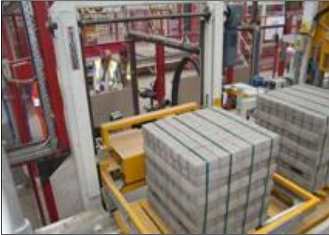
A Signode machine in operation strapping non-palletised concrete pavers using Signode Tenax® PET polyester strapping. Depending on the type of product the loads can also be lightly compacted or settled before strapping. Pallet loads of pavers can also be strapped by the equipment.
